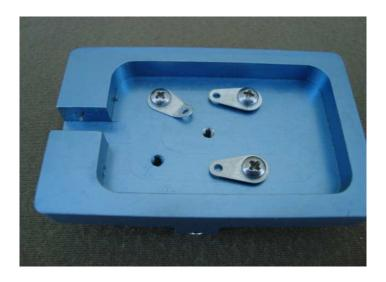
The other plain #4 x  $\frac{1}{4}$  pan head screw and flat washer secure the strain relief. The base is now ready to receive the levers.
