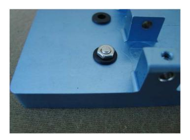
Slide the remaining solder lug over one of the plain #4 x  $\frac{1}{4}$  pan head screws, and thread into the base from the bottom into the grounding hole as shown. Note: The ground hole threads are not anodized!
