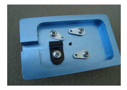
Next is to prepare the levers. Screw the shorter ground end  $\frac{1}{4}$  pan head screws into the holes nearer the paddle finger surface. Thread the thumb nuts onto the four thumbscrews, and screw them into the remaining two holes. Thread two standard nuts onto each of the end thumbscrews. With the bottom nut flush to the bottom of the thumbscrew, tighten the other nut to lock them to each thumbscrew.
